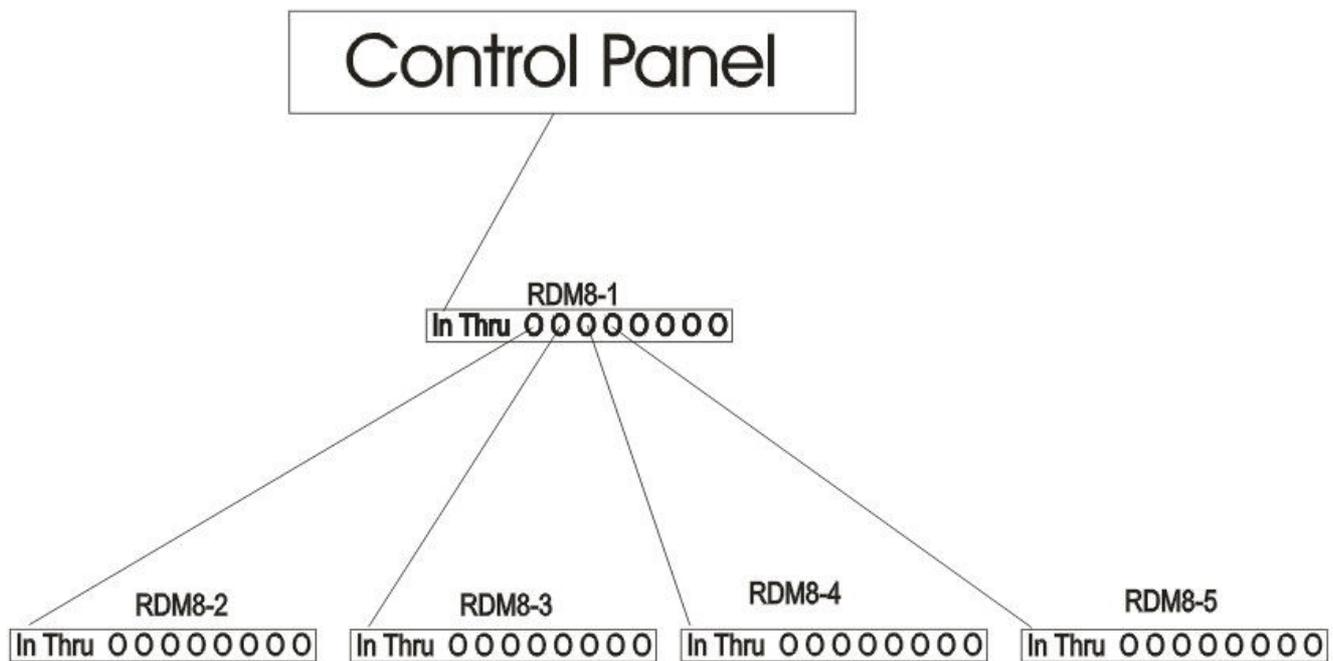
The star connection above provides 36 RDM outlets – any of which can then drive a normal RDM/DMX daisy chain of up to 32 RDM devices. More RDM8 splitters can be added, *so long as each RDM8 input is connected to another RDM8 output*. To avoid data clashes, do not connect any RDM devices (including RDM8s) to the RDM8 Thru output.
